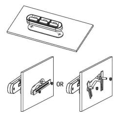
The rear of the switch is reversible so that the switch wire harness can exit the top or bottom of the switch housing.
