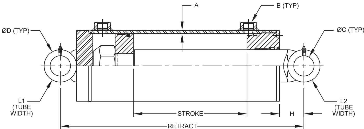
Rods are sized for a maximum safe push load (2:1 safety factor) given in the table. This is based on the pin configuration shown with no center support.
