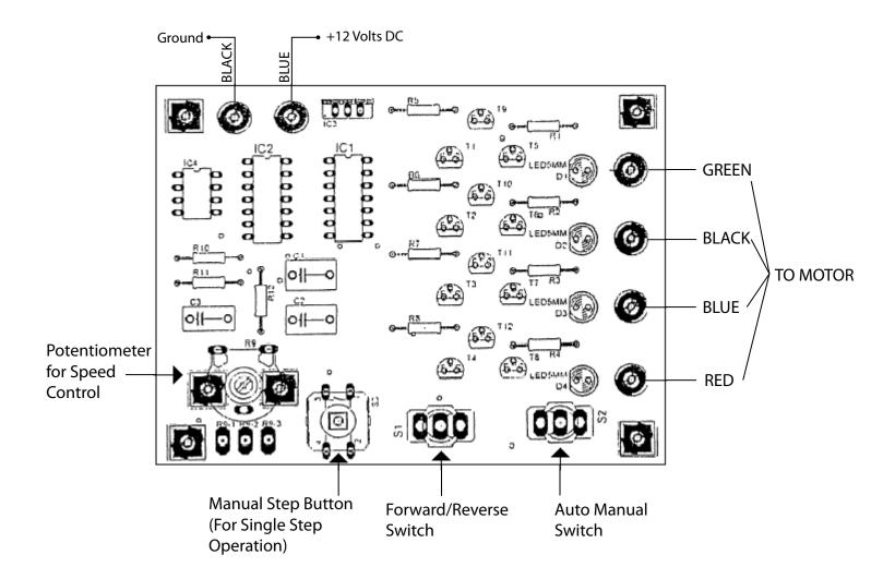
Incoming power connects to the BLUE and BLACK wires coming from the board. +12 volts DC connects to the BLUE wire, the BLACK wire connects to Ground.
