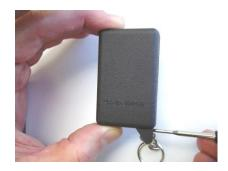
Carefully use a small screwdriver to pry open the case.
