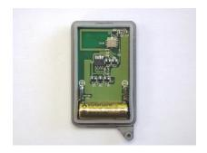
When replacing the battery, be sure to observe the noted polarity.
