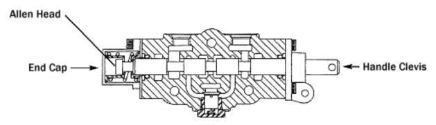
Before installing your joystick handle assembly kit, you must first remove the existing handle clevis end. As these are on very tight, the manufacturer recommends the following steps.
