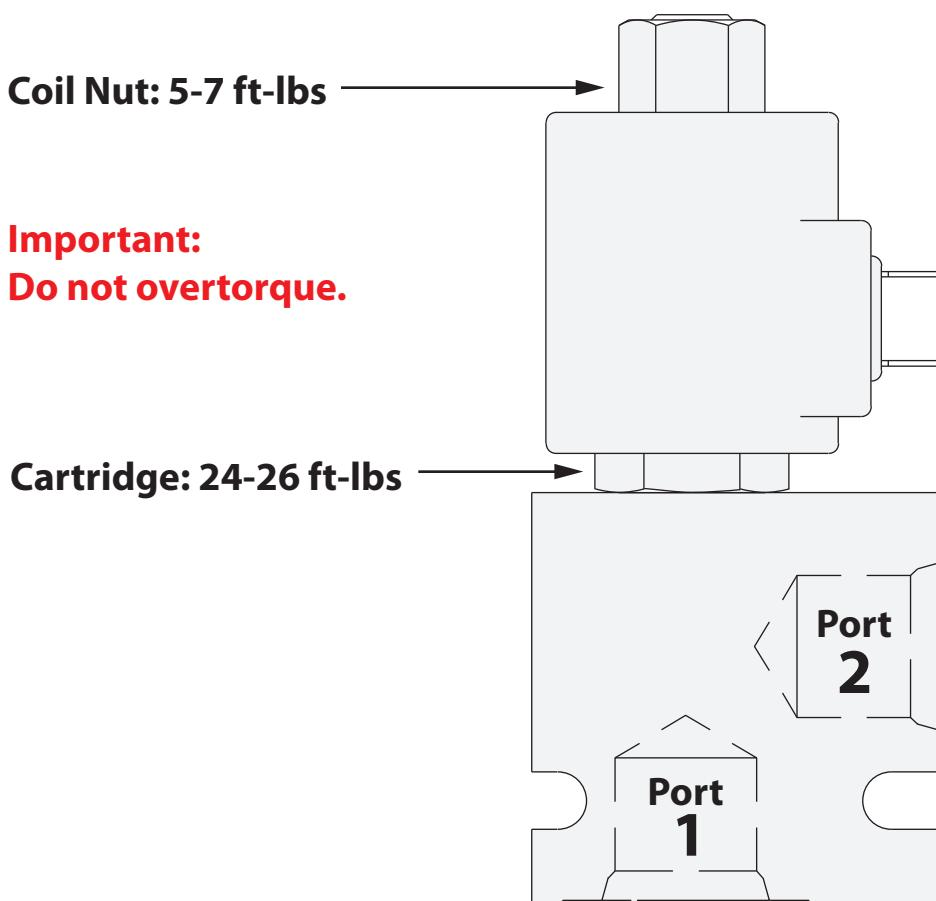
**9-5111-NO & 9-5112-NO:** When de-energized, the valve allows bidirectional flow from port 2 to port 1. When energized, the valve's poppet closes to block flow from port 2 to port 1. In this mode, the cartridge allows free reverse flow from port 1 to port 2, after overcoming the solenoid force (50-150 psi).
